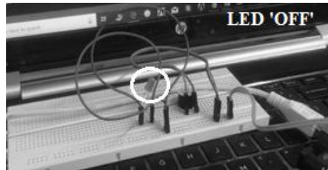
Fig. 6. Buzzer and LED light OFF during temperature within limit
