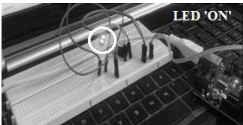
Fig. 5. Buzzer and LED light ON during temperature exceeding limit
