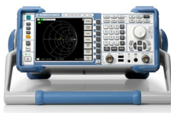
Vector Network Analyser operational upto 40GHz
