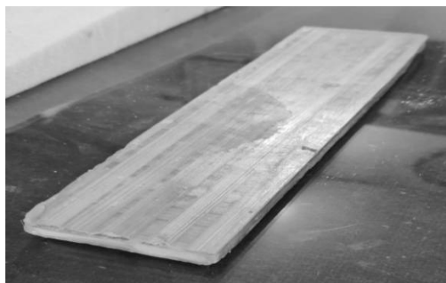
Fig. 2. Beam made with Bamboo epoxy skin and PU foam core
